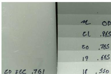
Programming the lamp delay time to 0.05 seconds results in the test strip on the left. 20 one second exposures now equal 1 20 second exposure.
