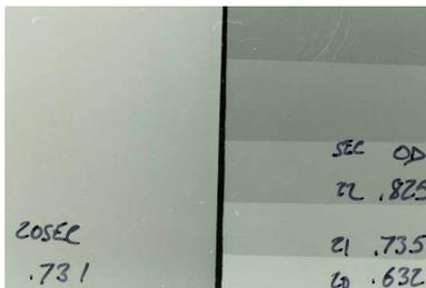
Match the density of the 20 second exposure to one of the test strips. In the example the matching strip is the one with 21 x 1 second exposures.
