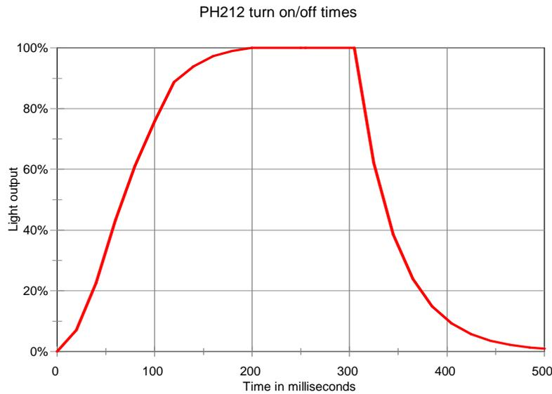
Lamp delay compensation with cold light heads can be problematic. The delay is affected by the lamp temperature and the time between exposures. A consistent pacing when making test prints is required for very accurate results.
